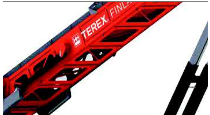
Discharge Conveyor Underguard
