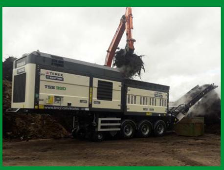
The TSS 390's 3m long shredding shaft was expertly designed in-house and is made from heavy-duty steel, with easily replaceable, bolt-on shredding teeth. Being hydrostatically driven, it offers the benefit of full speed, full torque reverse as well as protection against contaminants. Customisable shredding programs enable the operator to configure the machine to their specific requirements and offers improved shaft cleaning in difficult applications, reducing wrappage and optimising throughput.
