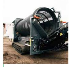
Easily replaceable 4.7m (15'5") x 1.8m (5'1") punch plate drum which is compatible with the Doppstadt SM 518
