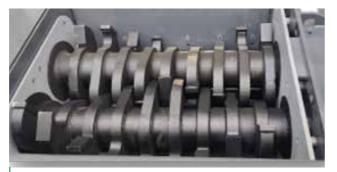
Expertly designed in-house shredding chamber 2 x 1.5m long shafts made from heavy duty steel with
