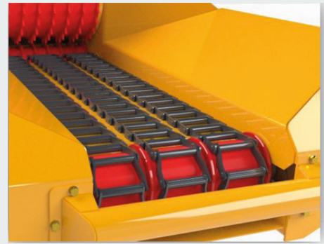
Infeed designed with 5" pitch chain. Bottom feed roll helps guide material to the rotor.
