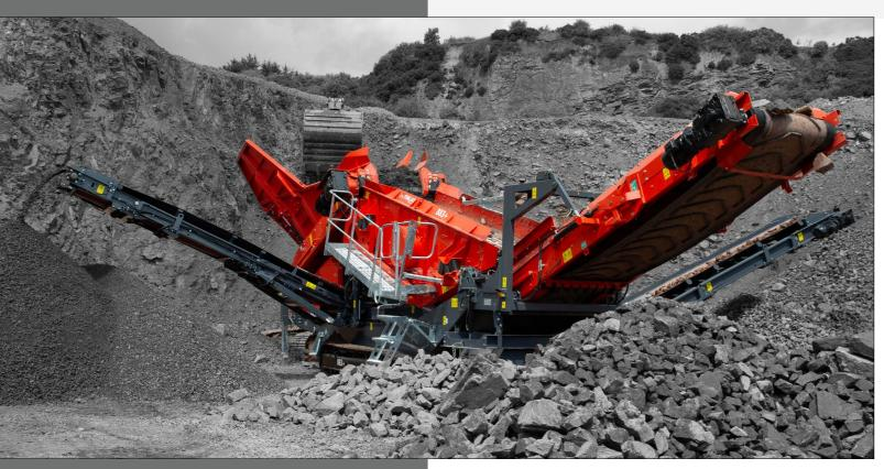
The Finlay® 883+ electric scalper has been designed to meet the needs of customers for whom electricity is the preferred power source. The intelligent and flexible design of the power pack enables the machine to be connected directly to the grid or a genset electrical power source.
