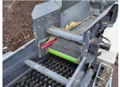
Fully adjustable metering wheel - speed, height & lateral position
