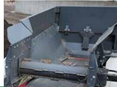
Hydraulic folding hopper extensions allows for increased capacity
