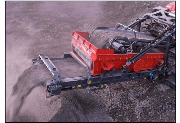
Main & Fines Conveyors
